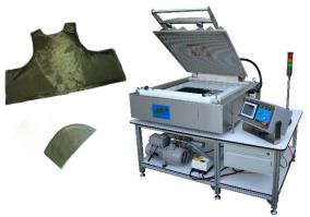
The **ASC BAIT** is an integrity test instrument for ballistic packs.
